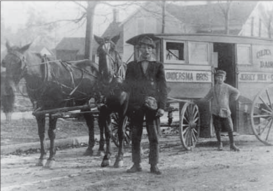
A wagon specifically designed for milk deliveries had a step-into driver's compartment that was much easier for the route man than the older carriage-style wagons that required climbing up in order to enter. The area in front of the driver area was waist high to facilitate sorting and assembling orders. The back of the wagon held the crates of milk loaded at the dairy that morning. Courtesy of Jacob "Bick" Ondersma.
