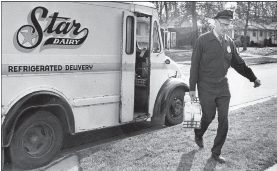
Horses stopped being used in the early 1950s. But Fred, seen here in 1978, continued delivering by truck until 1979. This step-in van by Divco (Detroit Industrial Vehicle Company) was specifically designed for delivery service. This milk delivery vehicle was refrigerated. Courtesy of Fred Ondersma.
